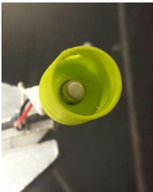
Figure 5. Unfinished sensor, transistor head can be seen within the 3D printed casing
